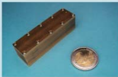
Power-generating cell stack
